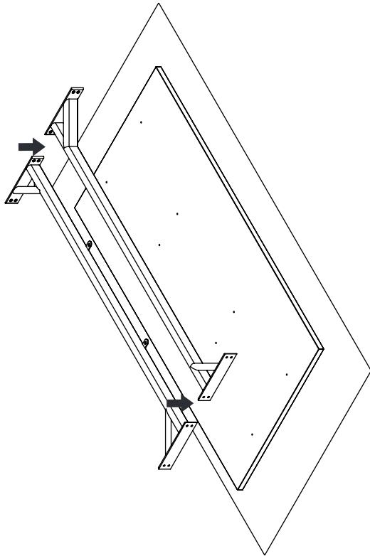
Use the allen key and this screw to fasten the rails
