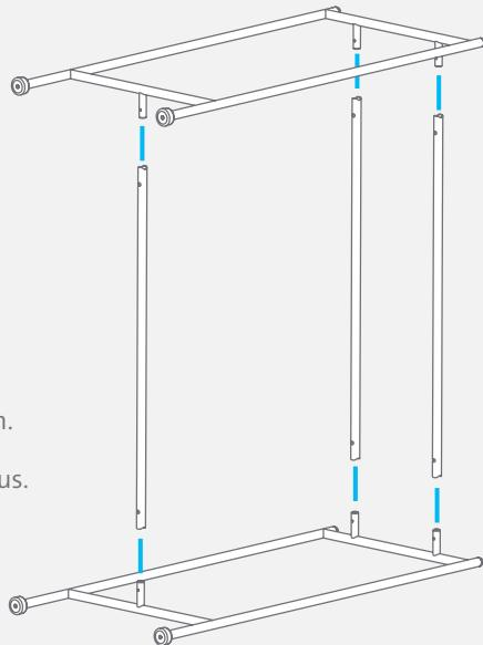
**EN** Align the holes towards the bottom.
