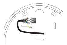
Plug the cable from the ceiling outlet into the terminal clamp and secure it with the strain relief.
