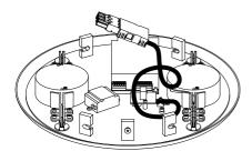
The assembly of this luminaire requires two people. Position the cable as pictured, before connecting the clamp, to ensure a flawless assembly.
