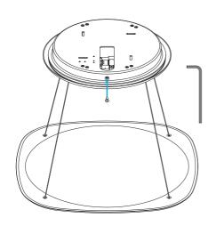
Tighten the screw to secure the ceiling fixture cover.
