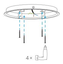
The installer is responsible for choosing the correct fasteners. The installation of this luminaire to sloped ceilings is not permitted.
