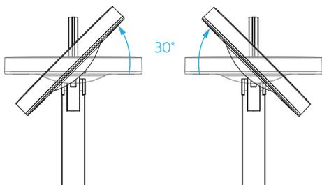
Please note the range of movement / angle of inclination of the lamp head joint.
