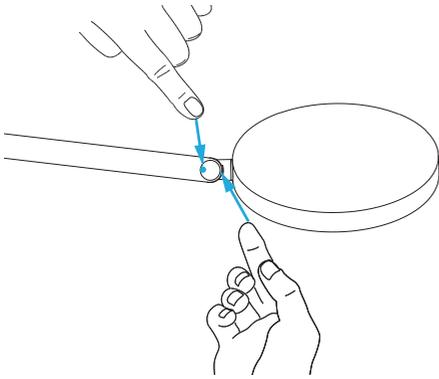
The lamp head joint can be readjusted using a small screw. To do this, carefully remove the cover plate over the joint and slightly tighten the screw with the allen key provided. Then replace the cover plate over the joint.
