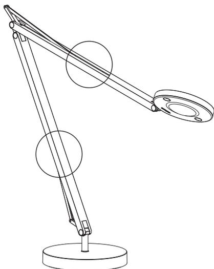
The force of adjustment of the lamp/ luminaire/light can be altered at a later stage. To allow for less mobility, tighten the screws by turning them clockwise at the marked points. To allow for more mobility, loosen the screws a little.
